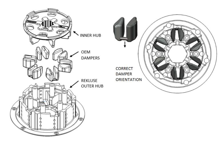
3. Install the new center hub assembly into the motorcycle.
