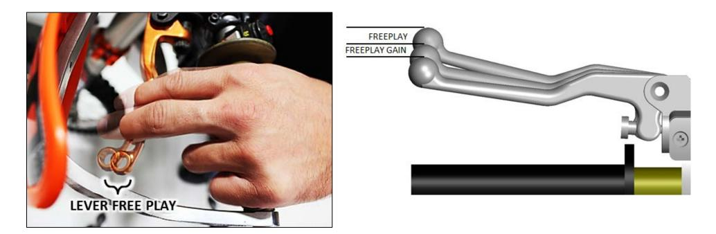
If there is too much Free Play Gain, the installed gap is too small. The bike may drag and stall because it has difficulty disengaging the clutch. It may also be difficult to shift. Too much Free Play Gain will not hurt the clutch, but it will negatively affect clutch performance.
