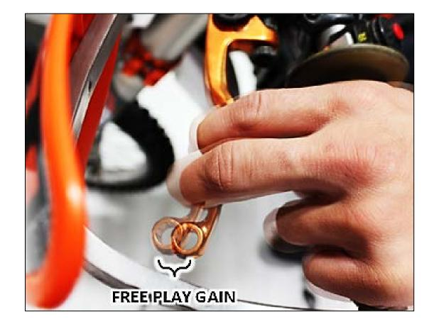
c) While still in **NEUTRAL**, continue to apply light pressure and quickly rev the engine between 5,000-7,000 RPM (1/2 to <sup>3</sup>/<sub>4</sub> throttle), then let it return to idle. Notice the movement in the clutch lever when the engine is revved. This is your Free Play Gain.
