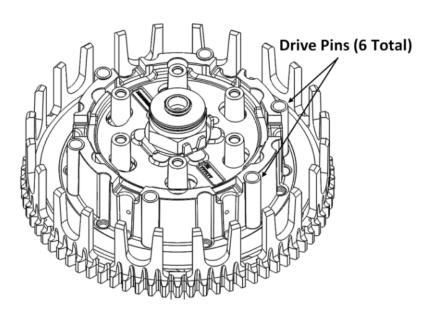
5. Use a hammer and large screwdriver to bend down the tabs of the washer tab, then remove the center clutch nut with an impact wrench or breaker bar, and a 27 mm socket.
