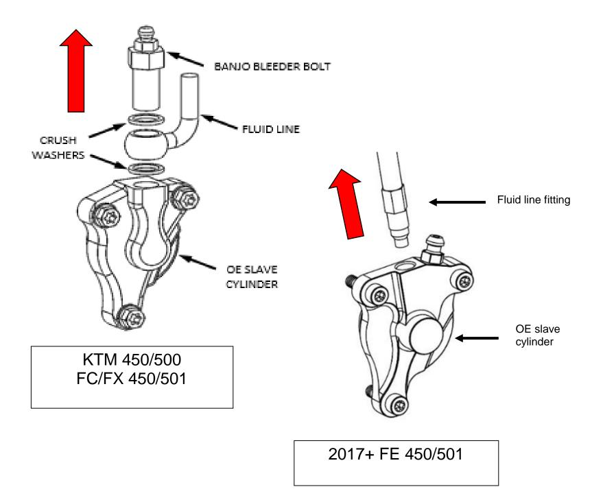
5. Attach the clutch fluid line to the Rekluse slave cylinder using the supplied banjo bolt and the 2 new crush washers from Rekluse.
