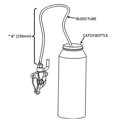
12. Pump the clutch lever 3-5 times then hold it against the bar/grip.
