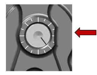
Tick marks are located on the slave cylinder, and an etch mark is on the screw. If you need to re-position the Allen wrench, you can use these marks for reference.
