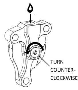
6. Use your thumbs to compress the piston again until it bottoms out while looking for air bubbles.
