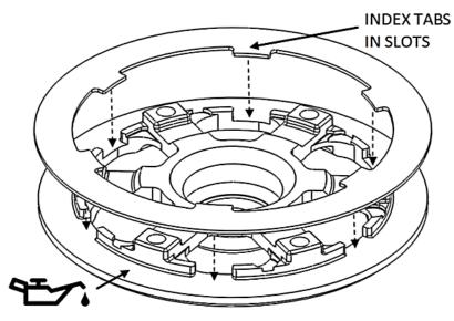
3. Install the pressure plate subassembly by lining up the index tabs on the pressure plate with the slots in the hub.
