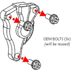
9. Mount the Rekluse slave cylinder to the engine using the OE bolts.
