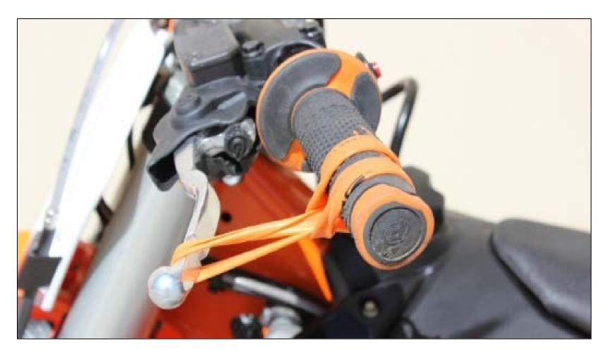
e) While still in NEUTRAL, quickly rev the engine between 5,000-7,000 RPM (1/2 to <sup>3</sup>/<sub>4</sub> throttle), then let it return to idle. Notice the movement in the clutch lever when the engine is revved. This is your Free Play Gain.
