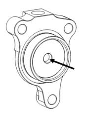
3. Pour the recommended clutch fluid into the slave cylinder port.
