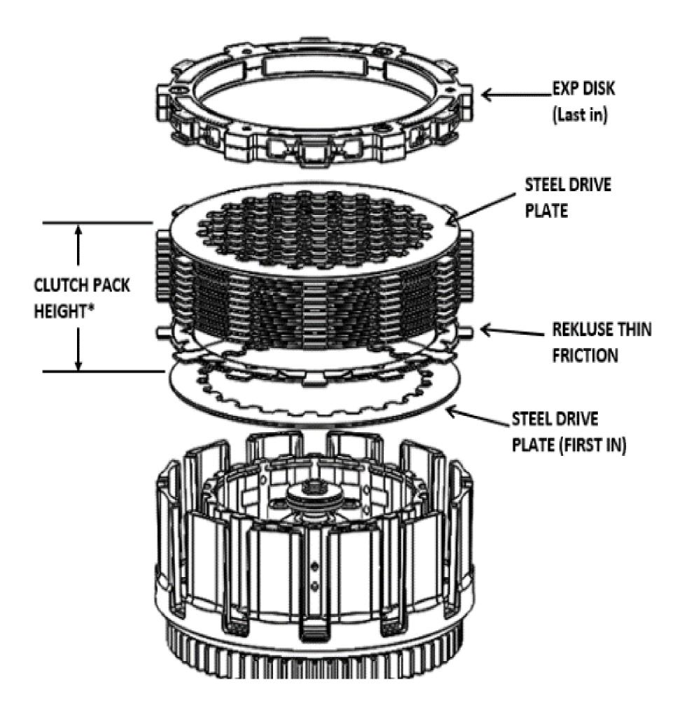
\*Refer to the Setup Sheet included with the clutch kit for the "Clutch Pack Height" specifications.
